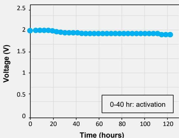
**Figure 1. Performance of AF2-HWP8-75 in 1M KOH and 80 °C:** polarization curve (top) and voltage at constant 1A/cm<sup>2</sup> for 120 hours (bottom)
