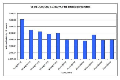
•Except for the 1min@150°C cure, volume resistivity performance of ECCOBOND CE3103WLV remains more or less constant at lower curing profiles. The material has a good conductivity in the 10-3/10-4 Ohm.cm range
