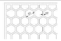
It is recommended to put more material in the location of possible hot spots and less material around the connection screws. This can be done by a denser honeycomb pattern in the locations where more material is required.
