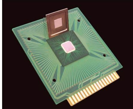
Based on a novel polymer PCM system, this material exhibits excellent wetting at interfaces during typical operating temperature ranges, resulting in very low surface contact resistance.
